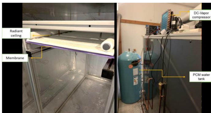
Figure 2: Laboratory equipment, radiant ceiling, water tank and DC-Vapour compressor
