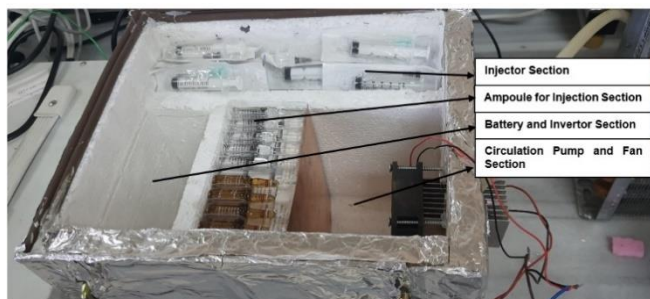
Figure 1: Schematic description of vaccine cabinet
