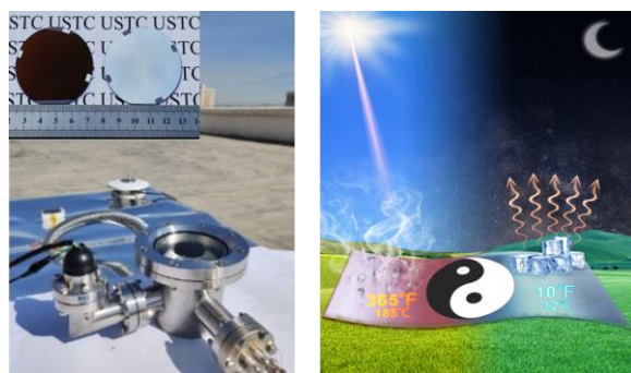
Figure 1: Al 2 O 3 /VO 2 /Al 2 O 3 /Al multilayer smart coating and its excellent diurnal solar heating and nocturnal radiative cooling performance.
